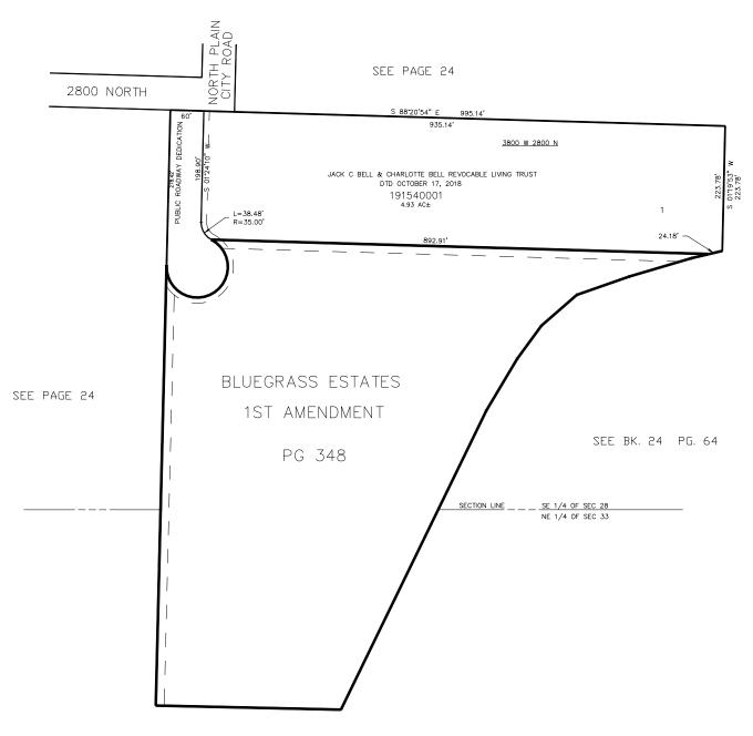
15' UTILITY & DRAINAGE EASEMENTS EACH SIDE OF PROPERTY LINES AS INDICATED BY DASHED LINES EXCEPT AS OTHERWISE SHOWN.
